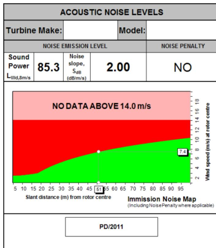
The noise map can be read by drawing a horizontal line from the recorded wind speed at the hub (right hand side of the map) to where the red and green lines meet. Drawing a vertical line from the point to the bottom of the map will give the maximum slant distance in metres from rotor centre (hub) at which a wind turbine could be installed to stay within the noise range. For clarity, MCS Contractors must draw a single line that is no greater than the thickness of a standard biro.
